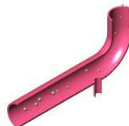
Fig.2. With heat, the particles decrease in size and all pass the bend in the Thermo-Split chamber.
