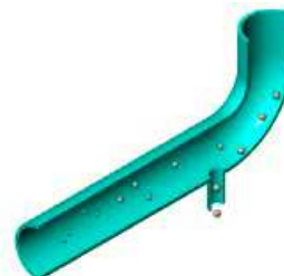
Fig.1.:With cooling, the particles condense and increase in size. They are carried into the walls of the bend and exit via the drain.
