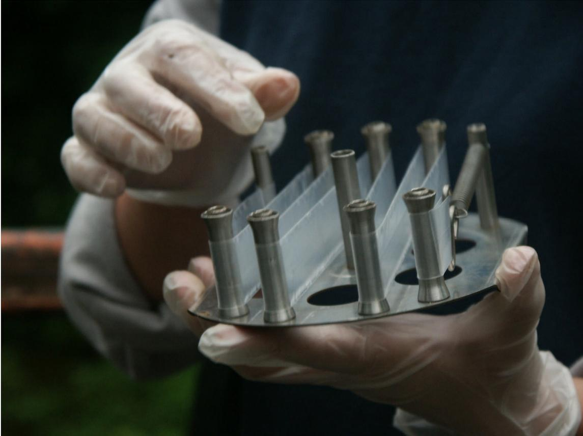
Standard size EAL mounted on the stainless steel spider
