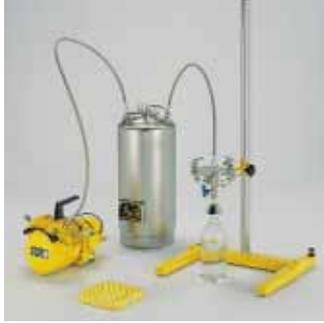
This holder is very often used in laboratories for particle removal and for sterile filtration of several liter volumes. It has a stable construction and is easy to operate. The large filtration area of 130 cm<sup>2</sup> ensures high flow rate for the total filter volume. The supplied unscrewable hose nipples can be replaced by G3/8 connectors, if systems with particularly practical handling is required.
