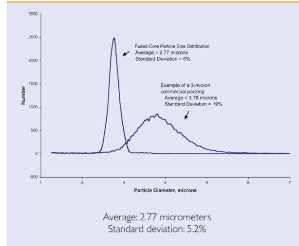
One of the distinguishing characteristics of Fused-Core particles is the unusually narrow size distribution compared to totally porous particles. This plot of particle number versus particle diameter illustrates how much more narrow the Fused-Core particle distribution is compared to typical totally porous particles.
