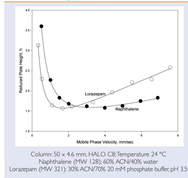
The unusually narrow particle size distribution plus the high density of Fused-Core particles, facilitate the packing of columns with remarkably good reduced plate heights,  $h$ . It has generally been assumed that a reduced plate height of 2 was the practical limit that could be achieved with packed columns and few commercial columns even achieve  $h$  values less than 2.5. The fact that columns
