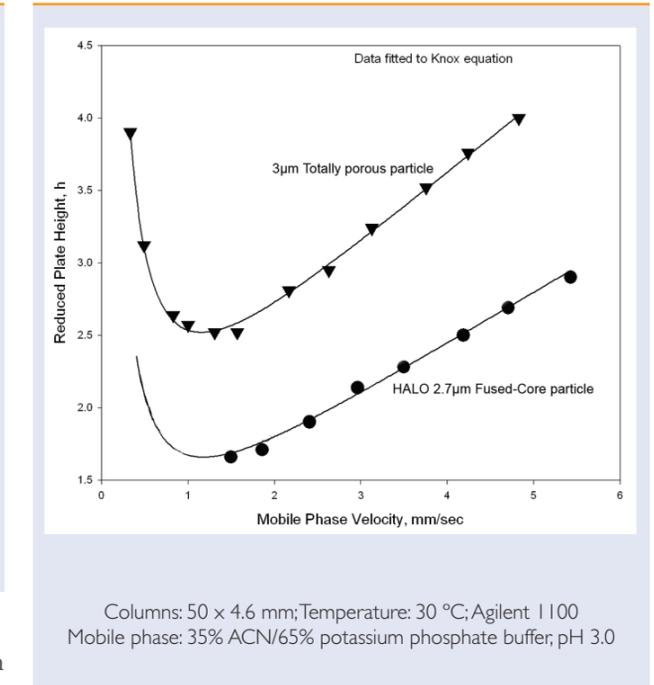
The short (0.5  $\mu\text{m}$ ) diffusion path offered by Fused-Core particles is particularly advantageous when separating larger size molecules. In this comparison of reduced plate heights for a column packed with 3  $\mu\text{m}$  totally porous particles and a column packed with 2.7  $\mu\text{m}$  Fused-Core particles (HALO), a solute with a molecular weight of 574 was used. The column packed with Fused-Core particles shows much superior reduced plate heights for this size molecule.
